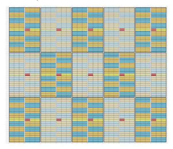
There are 15 total arrays (outlined in black), each having their own set of inverter skids (red cells). All of these inverters will feed the substation where power will be sent out to the grid.
