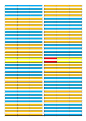
Each highlighted cell in the image above represents a rack of panels 25 modules wide and two modules tall. For each array, two racks will be removed to make room for the inverter skids bringing the total number of solar panels in each array out to 10,100.
